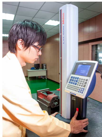
Measurement of inspection by 2D coordinate 2D
